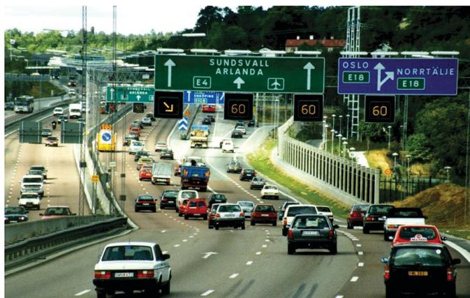
**Figure 3.2. Variable speed limit (VSL) control in Stockholm, Sweden.**
