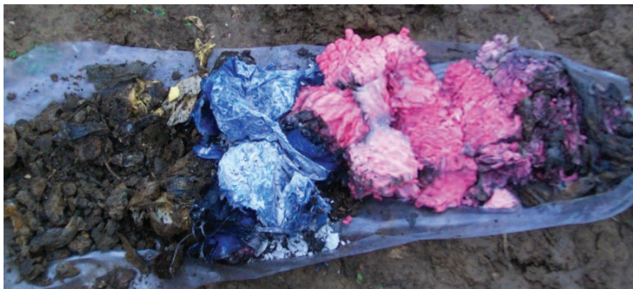
Typical roto sonic core of undegraded landfill waste and soil.
