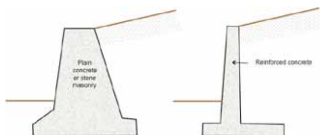
FIGURE 33 Cross section of gravity (left) and cantilever (right) retaining walls (Adapted from Das 2007).
