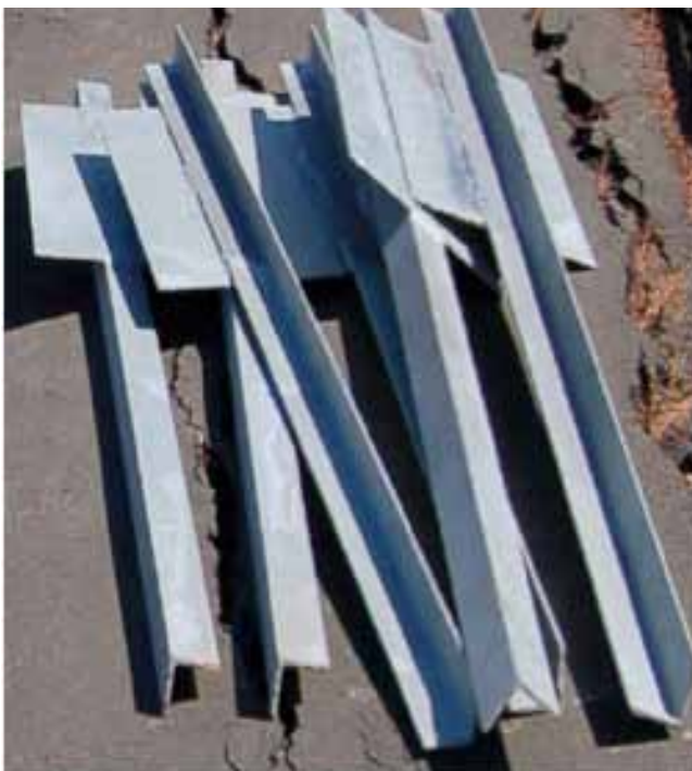
FIGURE 41 Six-foot plate piles (left) and plate pile installation (right) using an excavator with a hydraulic hammer (Courtesy: Y. Prashar).
