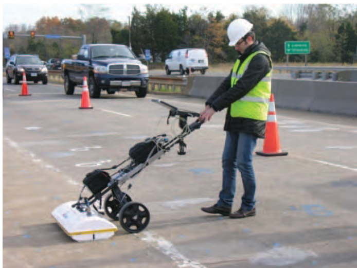
Figure 5.7. Ground-penetrating radar: IDS.
