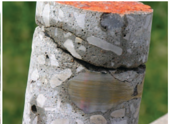
Figure 2.3. Corroded rebar in an excavated deck (top) and extracted core (bottom left), and delamination in a drill hole in a deck (bottom right).
