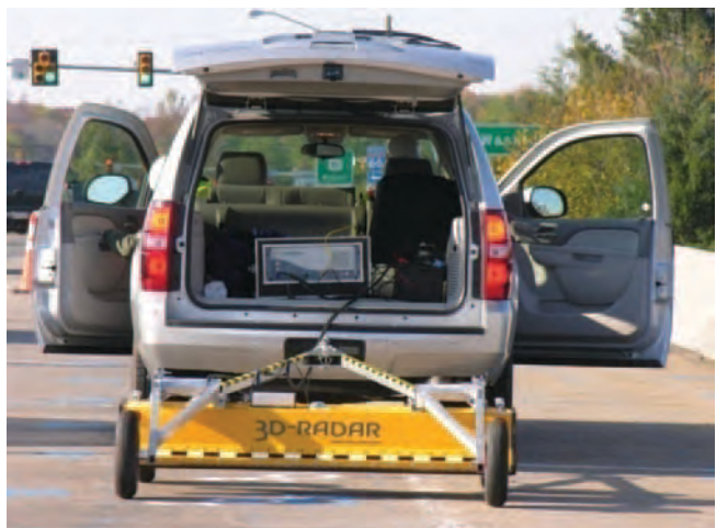
Figure 5.6. Impulse response (left): Germann Instruments. Ground-penetrating radar (right): 3D-RADAR.
