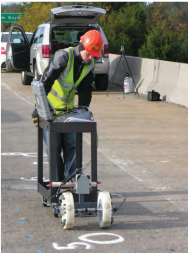
Figure 5.10. Impact echo and surface waves (left) and galvanostatic pulse measurement (right): Olson Engineering.
