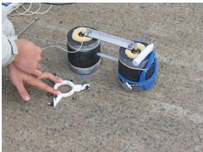
Figure 5.8. Air-coupled ultrasonic surface wave: University of Texas at Austin.
