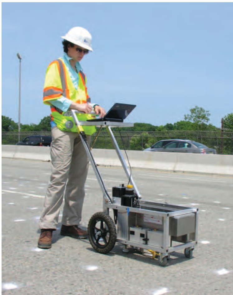
Figure 3.5. USW testing using a portable seismic property analyzer (PSPA).
