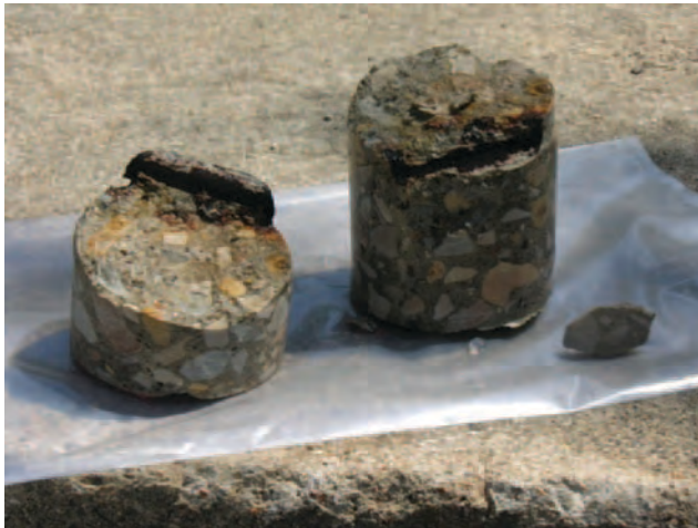
Figure 2.3. Corroded rebar in an excavated deck (top) and extracted core (bottom left), and delamination in a drill hole in a deck (bottom right).
