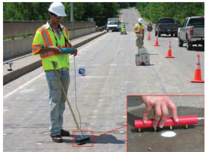
Figure 3.16. Electrical resistivity testing using a Wenner probe.
