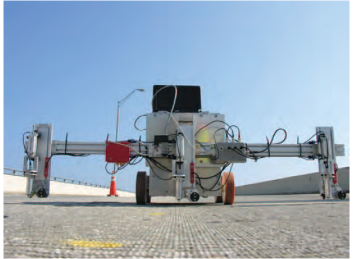
Figure 5.23. Impact echo (left): Olson Engineering. Impact echo (right): Rutgers University.
