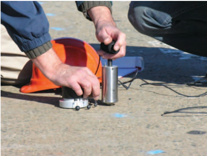
Figure 5.5. Impact echo: (left) Germann Instruments; (right) NDT Corporation.
