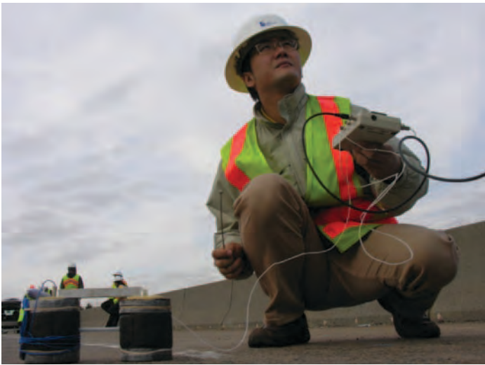
Figure 5.24. Air-coupled impact echo (left): University of Texas at Austin. Ground-penetrating radar (right): Rutgers University.
