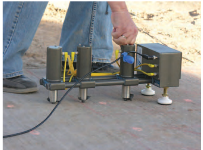
Figure 5.25. Infrared thermography (left): FHWA. Ultrasonic surface waves (right): Rutgers University.
