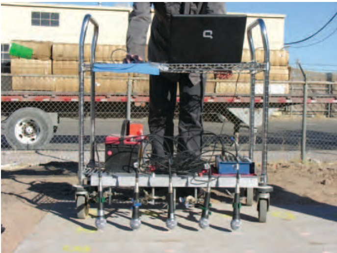
Figure 5.22. Air-coupled impact echo (left): University of Illinois. Impact echo (right): NDT Corporation.
