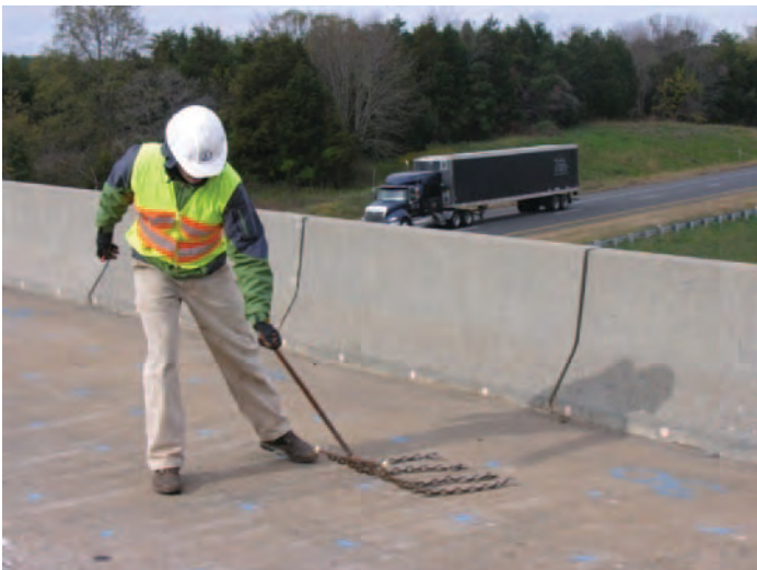
Figure 3.21. Chain dragging (left) and hammer sounding (right).
