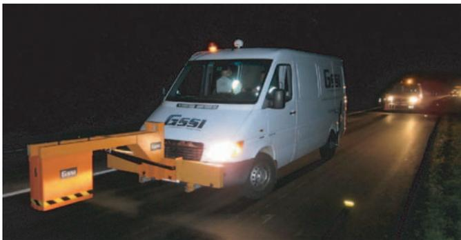
**Figure 3.74. GPR data collection for Region 1 demonstration.**
