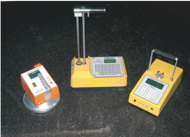
**Figure 3.26.** PQI, nuclear density gauge, and Pavetracker Plus.
