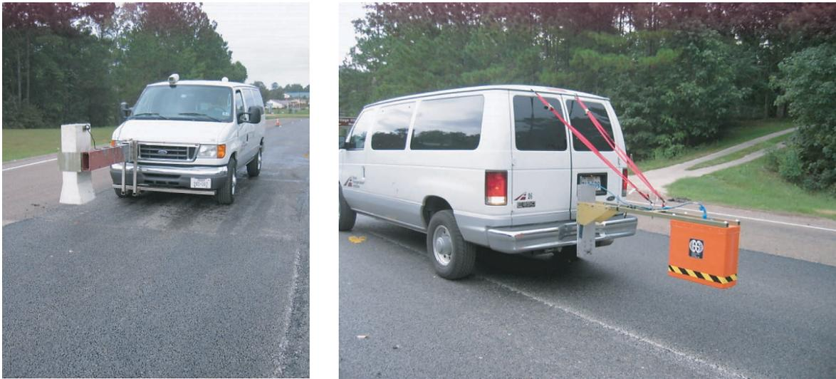
**Figure 3.37. 1-GHz (left) and 2-GHz (right) GPR data collection.**
