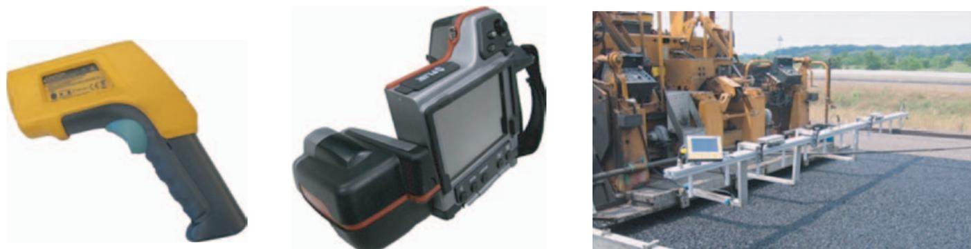
**Figure 3.4. Spot radiometer, IR camera, and IR bar measurement systems.**
