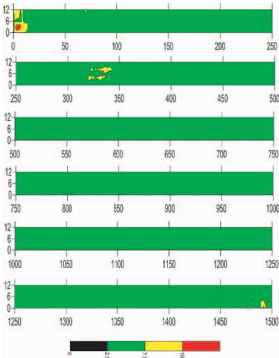
**Figure 3.80. Geospatial distribution of air voids on Region 1 project from 2.2-GHz radar.**
