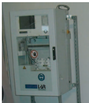
Figure 3.3. Example of an online monitor: a TOC monitor.
