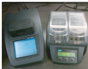
Figure 3.2. Example of a test kit: a COD digester.
