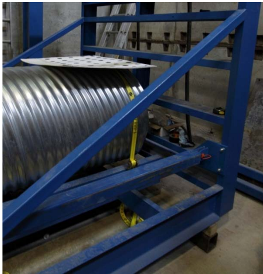
Figure H.8 End of loading frame on timber support. Figure H.9 Curved load plate and column.
