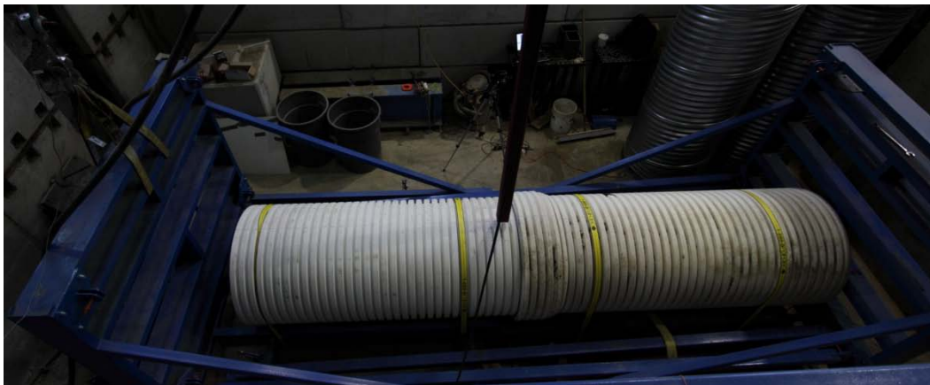
Figure H.12 The left hand end of the frame is held level then lowered for rotation testing of the PVC pipe.
