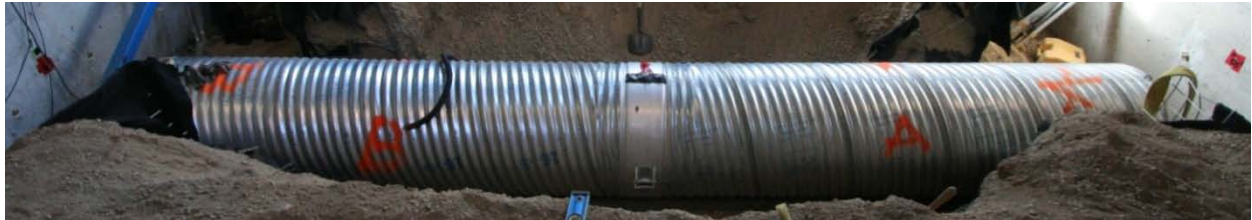
b. 36 inch (0.9m) diameter corrugated steel pipe with unsealed band joint
