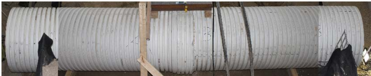
d. 36 inch (0.9m) diameter PVC pipe with gasketed bell and spigot joint
