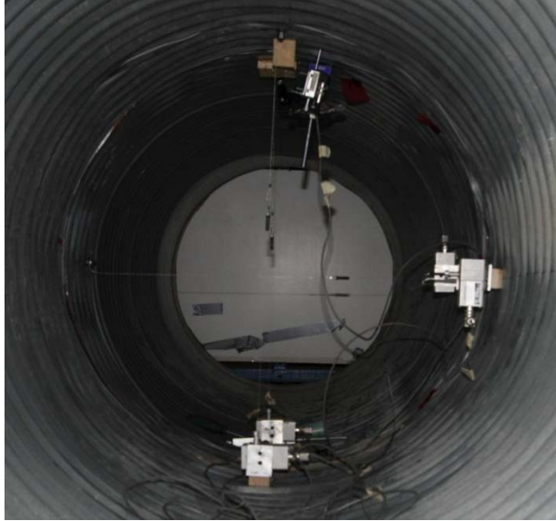
Figure H.10 Instrumentation used during shear testing of the corrugated metal pipe.
