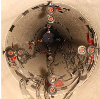
Figure C.9. View of the prisms after placement in the 24 in (610mm) diameter reinforced concrete pipe.
