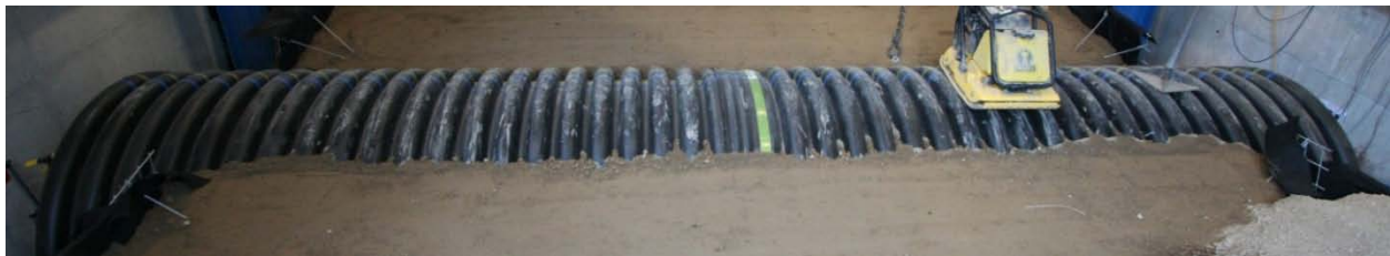
c. 60 inch (1.5 m) diameter high density polyethylene pipe with bell and spigot joint
