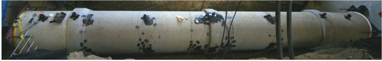
a. 24 inch (0.6 m) diameter reinforced concrete pipe with gasketed bell and spigot joint
