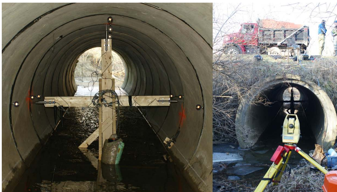
a) Instrumentation setup inside the culvert
