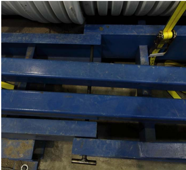
Figure H.11 Pin inserted for moment and rotation testing of the PVC pipe.
