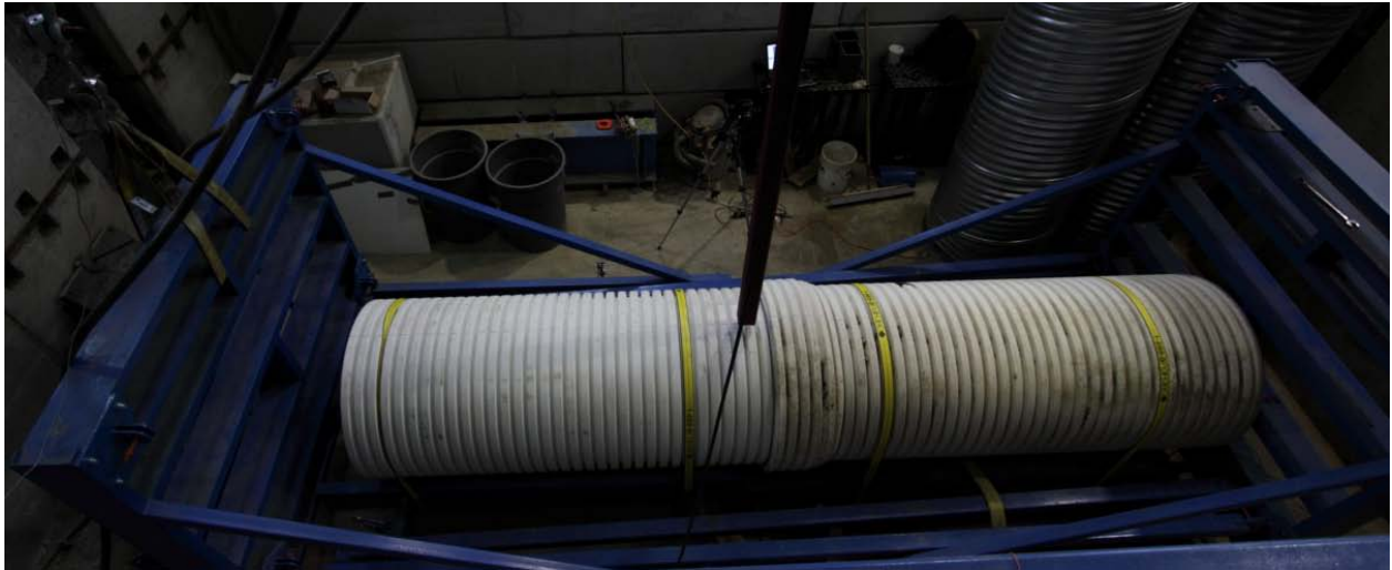
a. Configuration of the bending test on the PVC pipe; hinges are installed connecting the two frames under the joint and the left hand end is held and lowered to induce bending.
