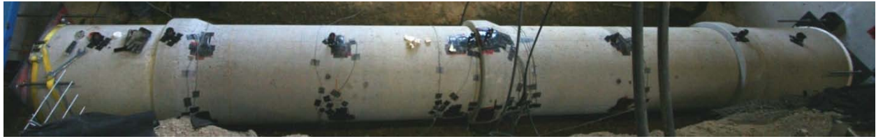
a. 24 inch (610mm) diameter reinforced concrete pipe with gasketed bell and spigot joint
