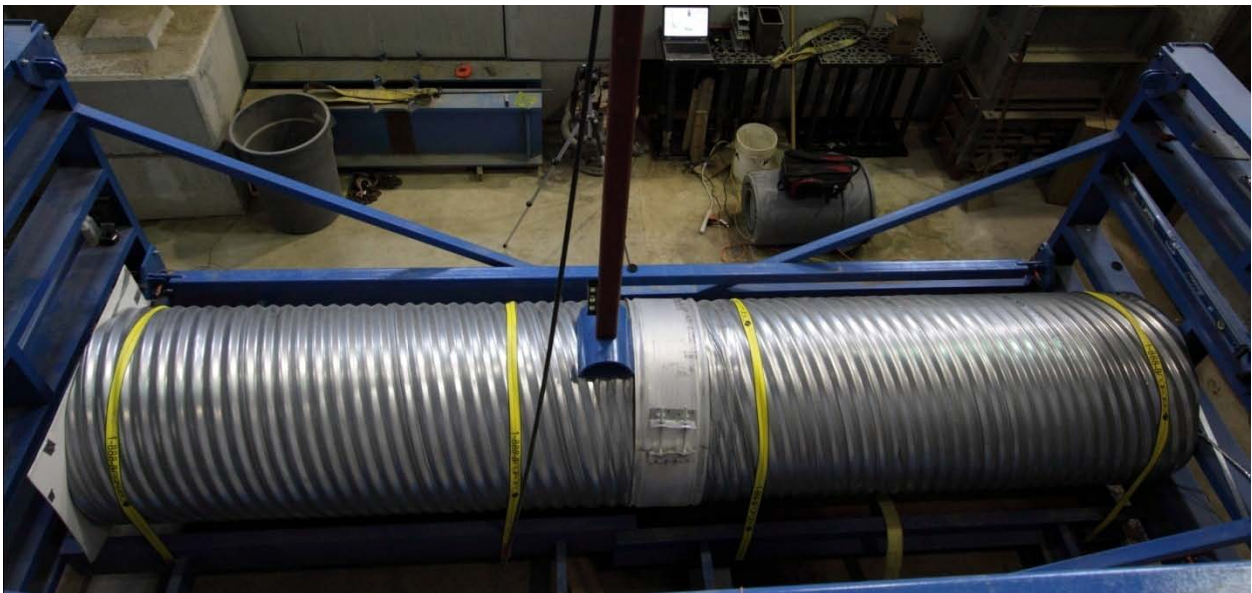
Figure H.5 Test frame (top view); this image shows the frame without the additional longitudinal ties; this configuration is used when testing joints without internal fluid pressure or vacuum.
