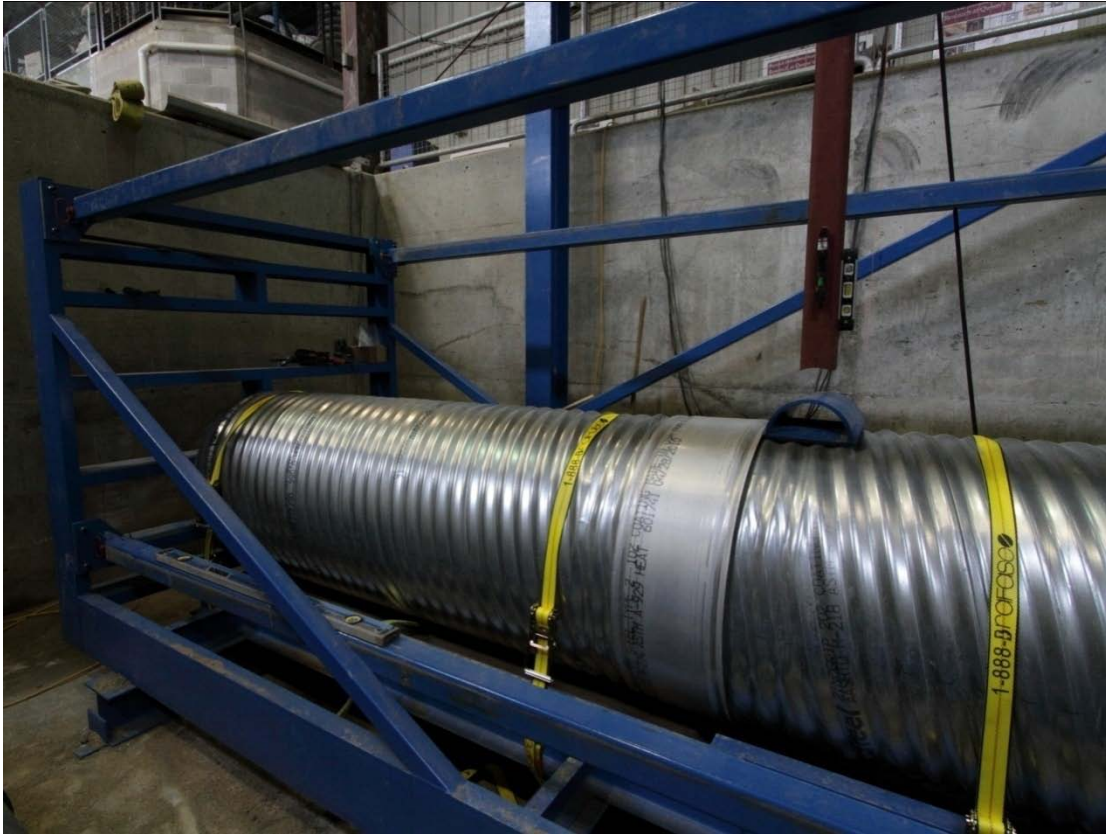
Figure H.4 Test frame in position for shear force testing; this arrangement shows additional longitudinal ties connecting the top corners of the end frames; these ties carry end reactions when sealing plates cover the pipe ends, these are tied to the end frames, and pipe has internal pressure or vacuum (future project).
