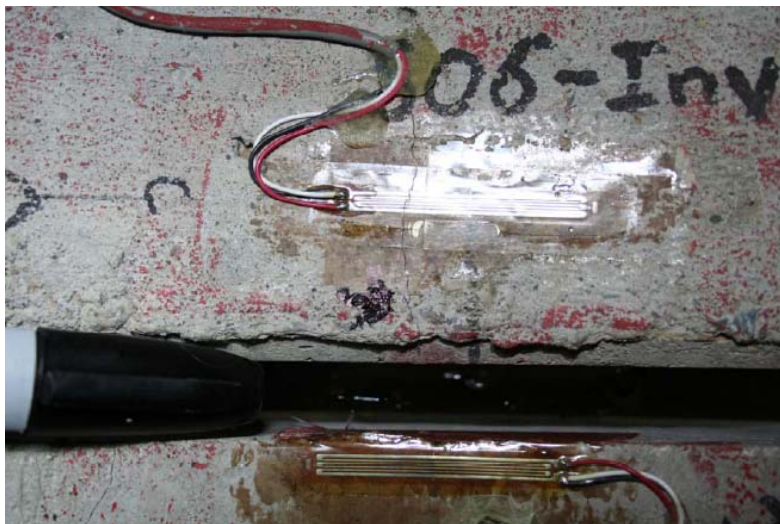
Figure C.26. Close-up of the invert of the 24 in. (610mm) diameter reinforced concrete pipe at the central joint; the joint is open about 1 in (25mm).
