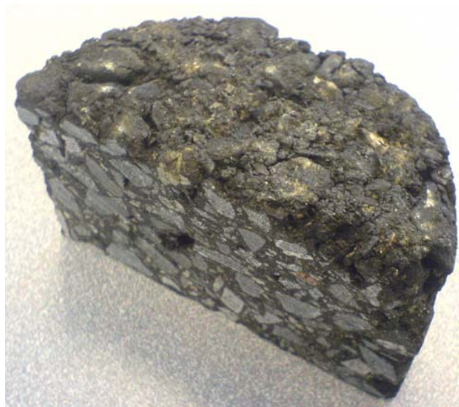
FIGURE 7 Mix manufactured with microalgae oil, using oedometric compaction system.
