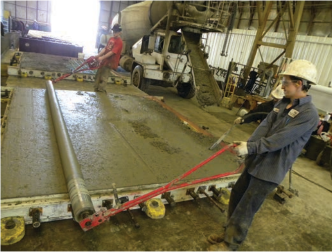
Figure 9.7. Placement processes for slump concrete and SCC.
