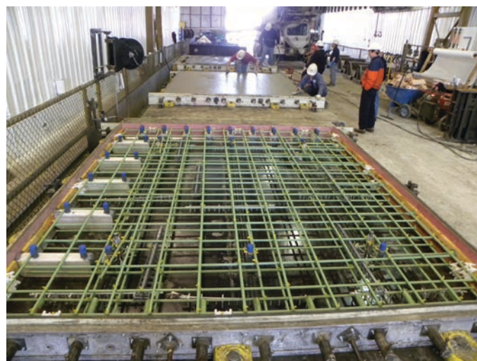
Figure 9.3. Reinforcement placed in both directions.
