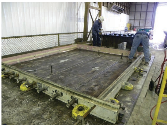
Figure 9.1. Typical formwork used for a continuous jointed PCP system.
