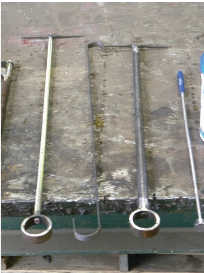
Figure 14.10. Tools to facilitate sliding the dowel bars in the slots and holding the bars in place.
