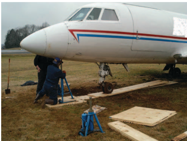
FIGURE 5 Jacking an aircraft. Source: Anonymous. Used with permission.
