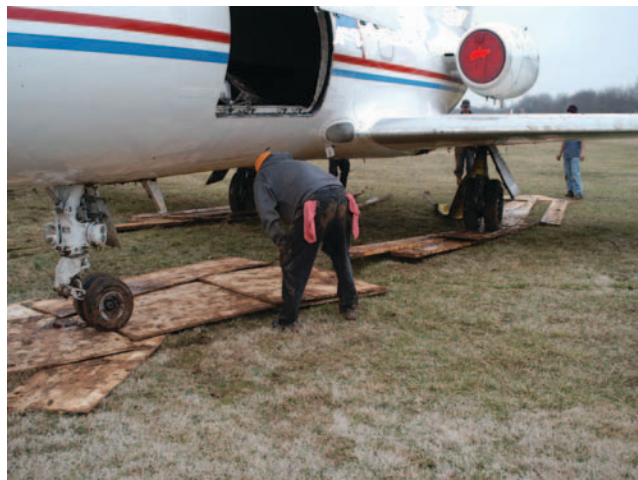
FIGURE 6 Temporary roadway in place. Source: Anonymous. Used with permission.
