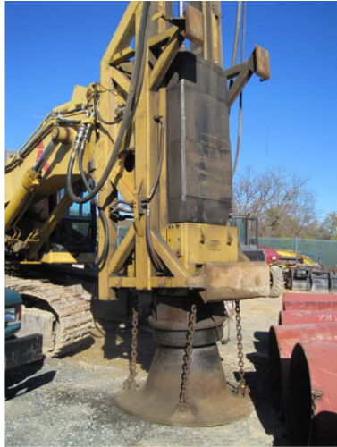
Hammer and anvil portion of rapid impact compactor. From the files of P. Becker.
