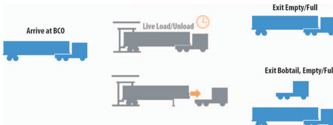
Figure 2-9. Chassis Operations at the BCO's Facility
