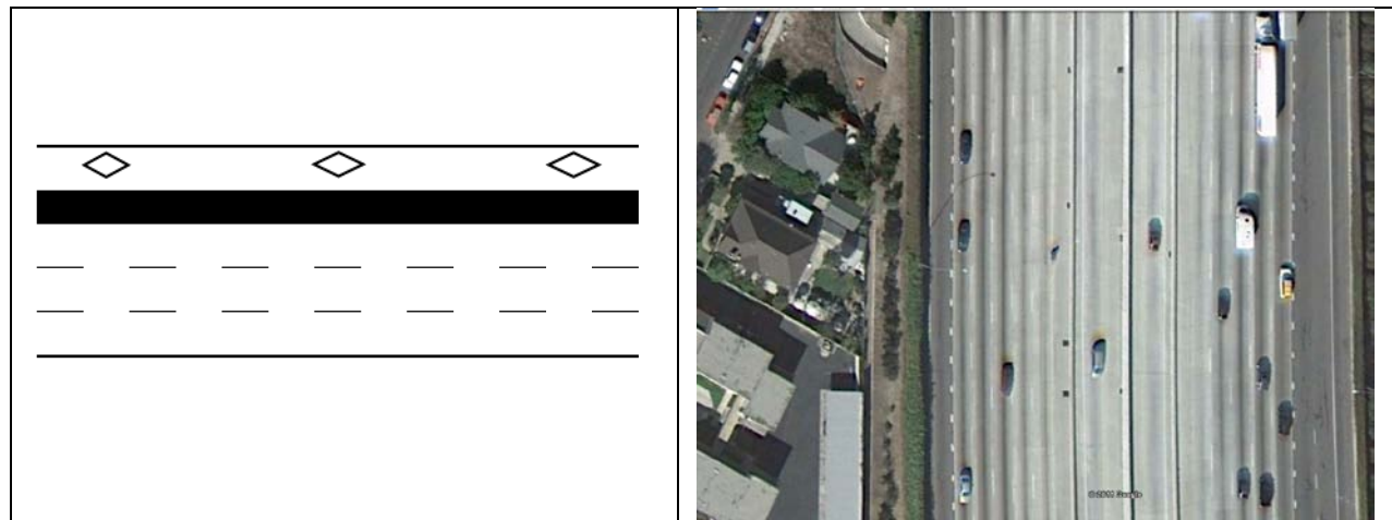
FIGURE 8 Schematic of Barrier 1 and Example at I-5 Orange County, California (Source: Google Earth)
