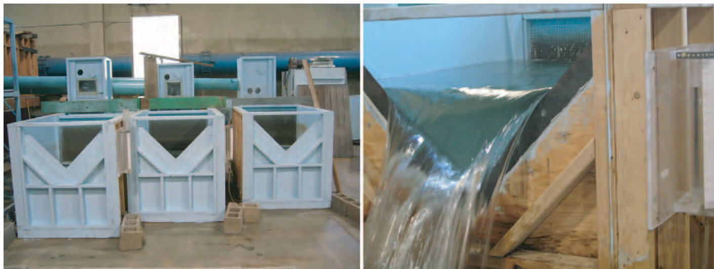
Figure 5-3. V-notch weir/tail box assemblies.
