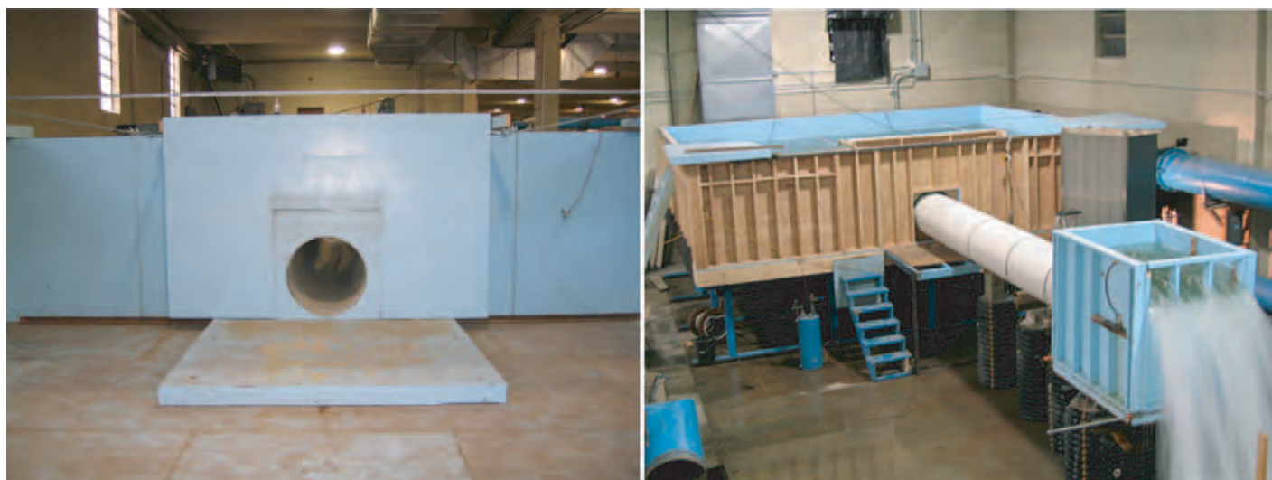
24-in. circular culvert
