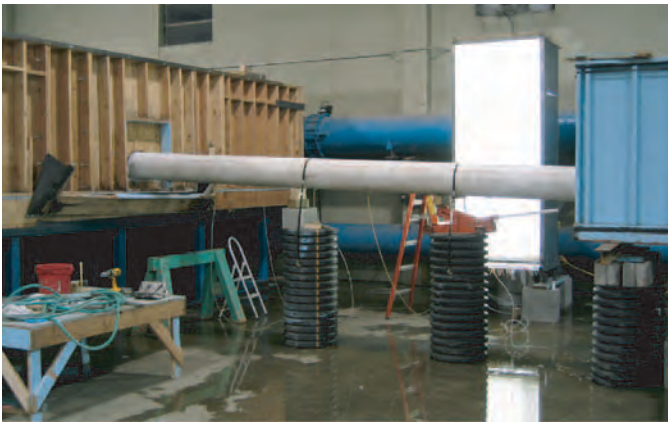
Figure 3-5. Overview photo of the culvert test setup.
