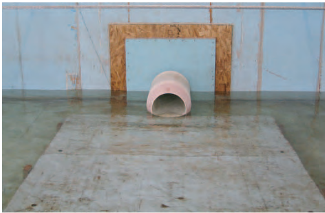
Figure 3-3. Ponded approach flow condition.
