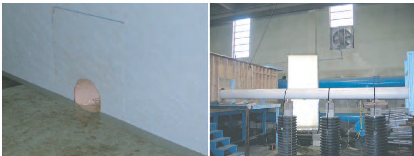
12-in. circular culvert
