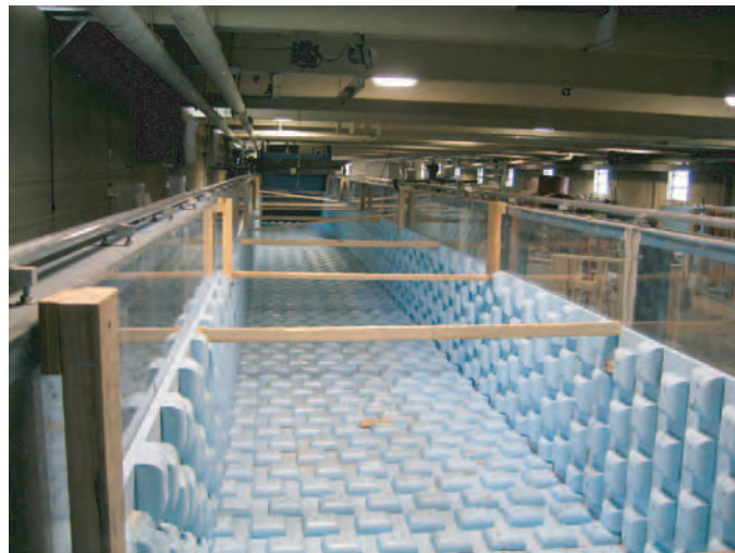
Figure 6-4. Block boundary roughness material.
