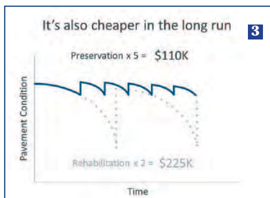
3 The theme of this slide, that preservation is cost effective, is a point that DOT executives care about.
