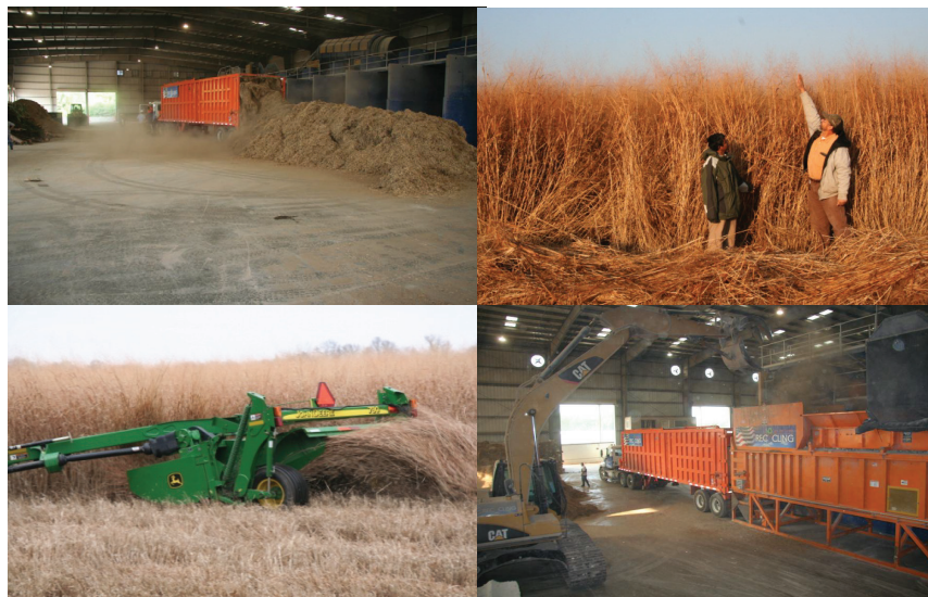
FIGURE 2-3 Bulk-format system to harvest, handle, store, and deliver low-moisture switchgrass. SOURCE: Image taken from Stokes presentation.
