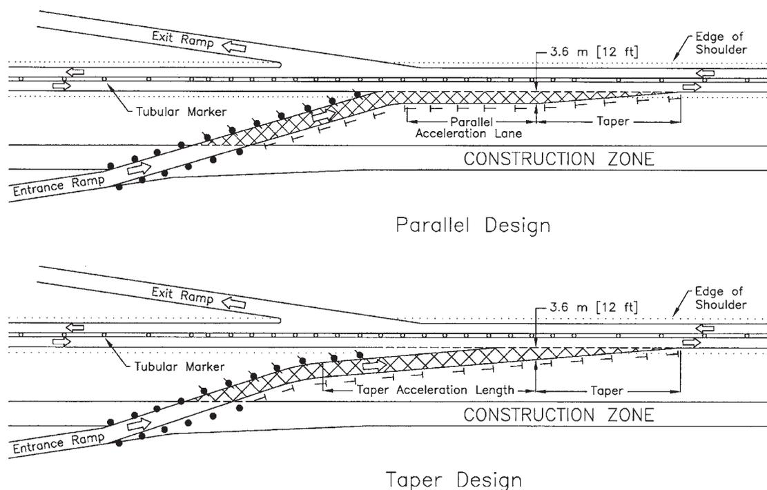
FIGURE 24 Temporary interchange entrance ramp for median crossover (Mahoney et al. 2007).
