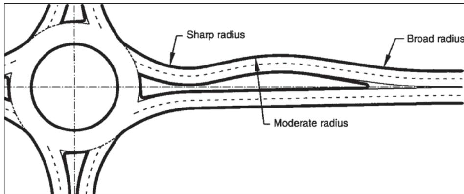
FIGURE 9 Example of approach curvature (Robinson et al. 2000).
