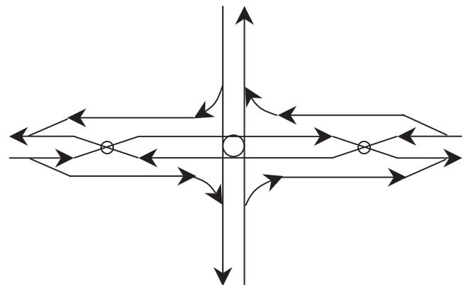
FIGURE 17 Double crossover intersection (Bared et al. 2005).
