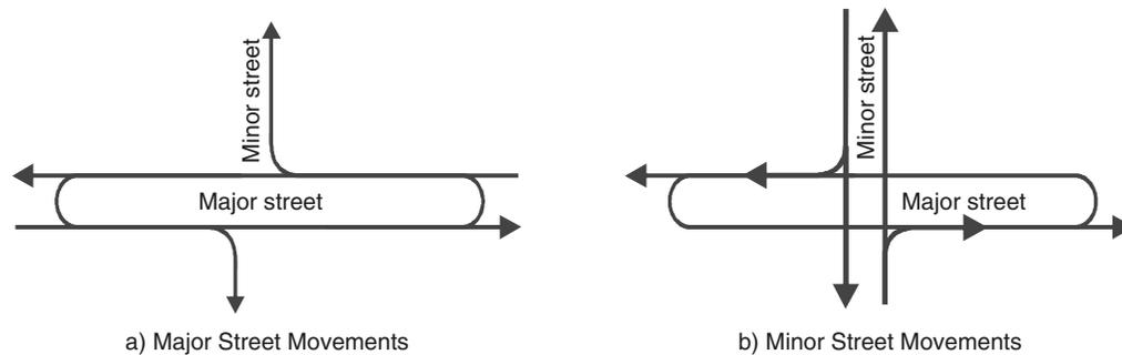
FIGURE 13 MUT left-turn movements (based on Hughes et al. 2010).
