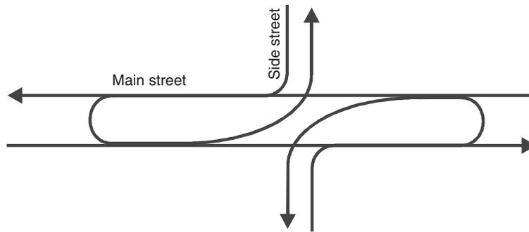
FIGURE 14 Conceptual RCUT configuration with direct left turns from the major road (based on Hughes et al. 2010).
