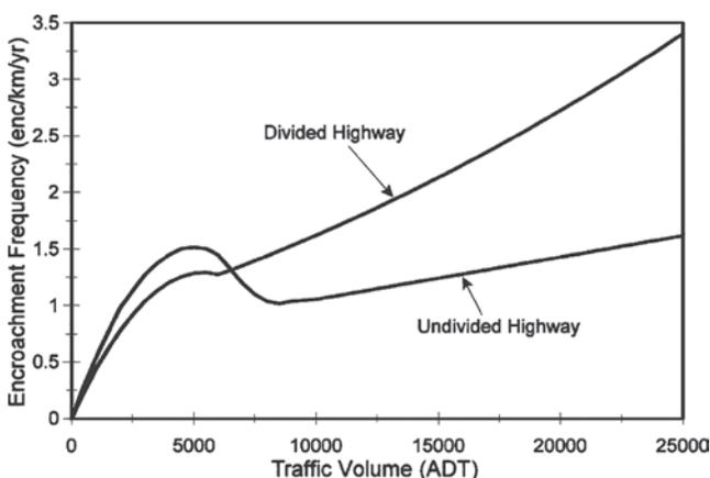
FIGURE 6 Encroachment rates used in Roadside Safety Analysis Program (Mak and Sicking 2003).
