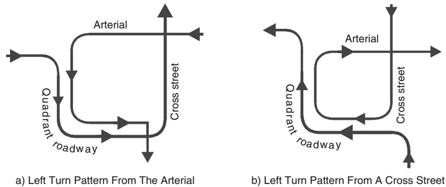
FIGURE 16 Left-turn movements at a QR intersection (based on Hughes et al. 2010).
