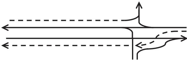
FIGURE 23 Detailed view of movements and paths for half of a DLT interchange.
