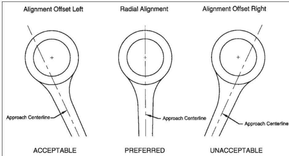
FIGURE 10 Radial alignment of roundabout entries (Robinson et al. 2000).
