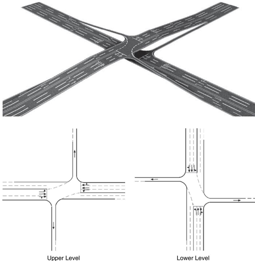
FIGURE 19 Concept design of two-level signalized intersection (Shin et al. 2008).
