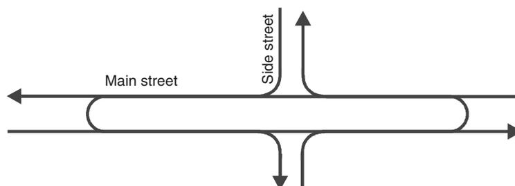
FIGURE 15 Basic RCUT intersection with no direct left turns (based on Hughes et al. 2010).
