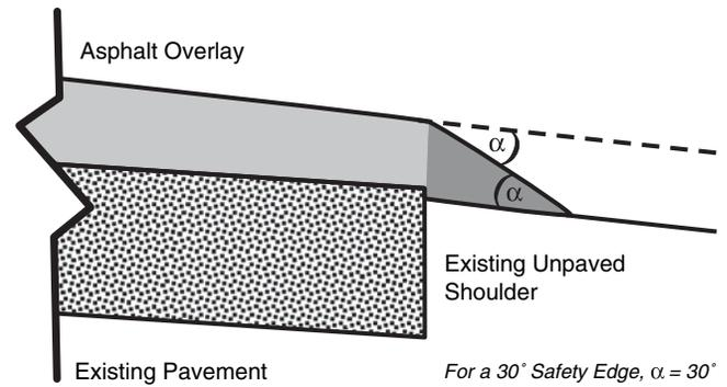
FIGURE 5 Illustration of FHWA's Safety Edge Treatment (Hallmark et al. 2006).
