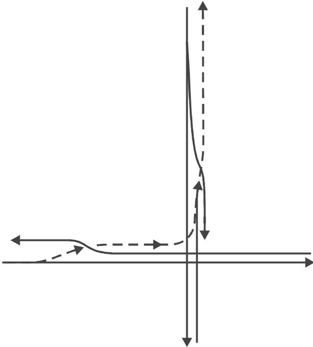
FIGURE 12 Left-turn movement on a typical DLT intersection approach (eastbound to northbound).
