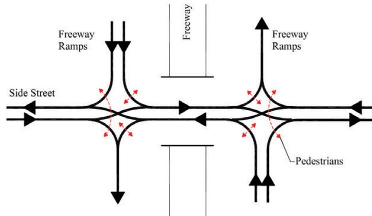
FIGURE 22 Typical DCD interchange configuration (Hughes et al. 2010).
