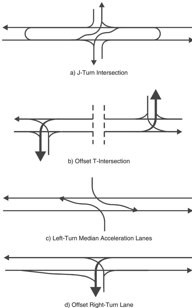
FIGURE 18 Diagrams of median intersection designs on rural expressways (based on Maze et al. 2010).
