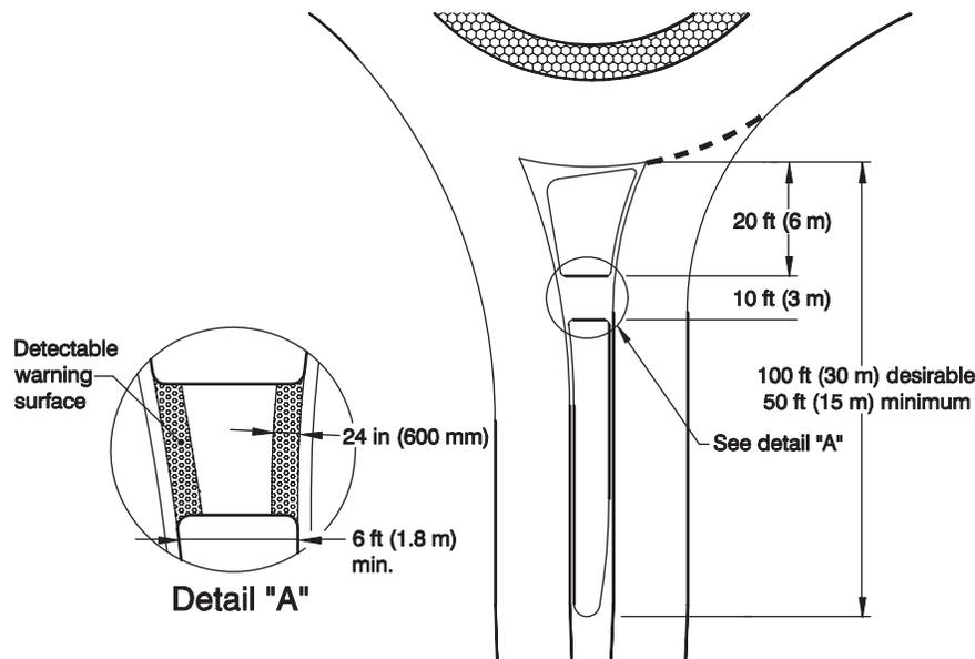
FIGURE 11 Minimum splitter island dimensions (Rodegerdts et al. 2010).
