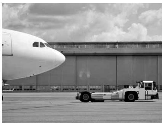
Towbarless tractor after disengaging from an aircraft nosewheel.
