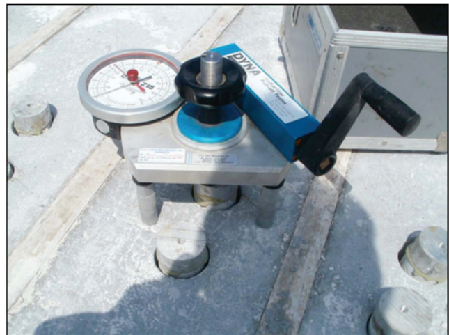
FIGURE 2 Apparatus for performing pull-off test to evaluate surface preparation or overlay bond strength.
