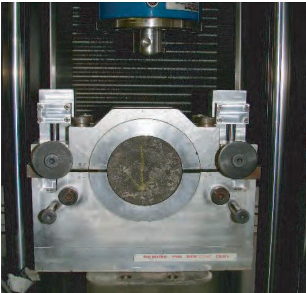
(c) Stabilization of test temperature (30 min.)
