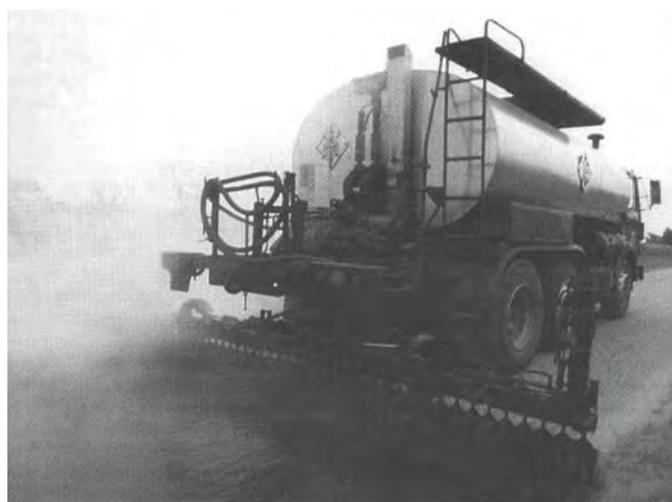
**Figure 4.** A typical asphalt distributor (courtesy of Etnyre).
