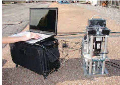
(h) Pull-off testing and data recording
