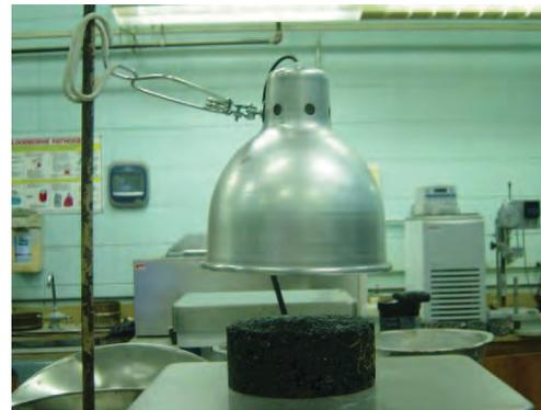
(a) Infrared reflective heating (IRH) lamp.
