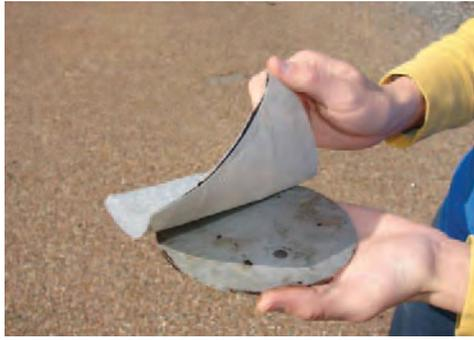
(e) Foam material attachment on loading plate
