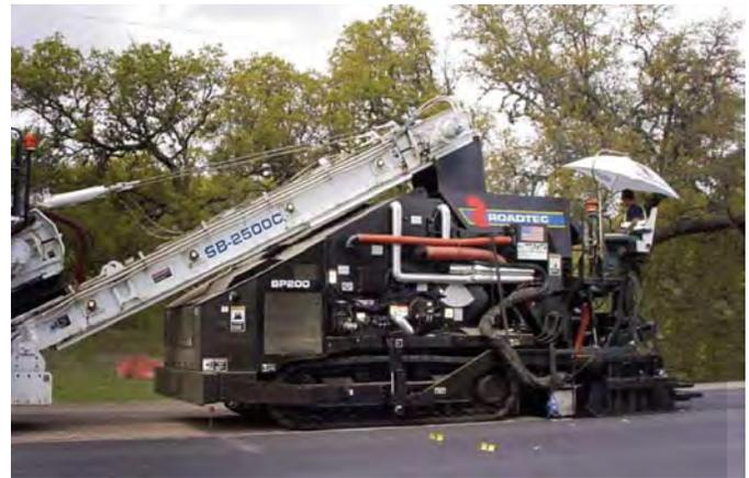
**Figure 23a.** Roadtec Spray Paver-Spray bar is located at white square between track and screed.
