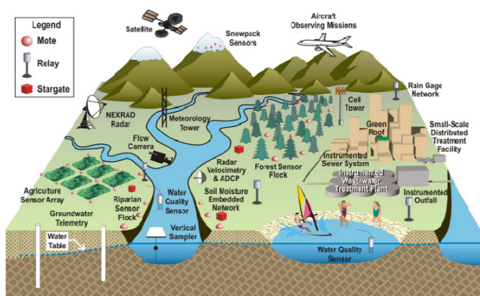
FIGURE 3-3 Schematic of an instrumented watershed in an observatory of the national network. Real-time sensors for meteorology, rainfall, stream velocity, suspended sediment, water quality, soil moisture, groundwater, and snowpack are shown with wireless communications equipment necessary for transmitting the data. Source: WATERS Network 2009.
