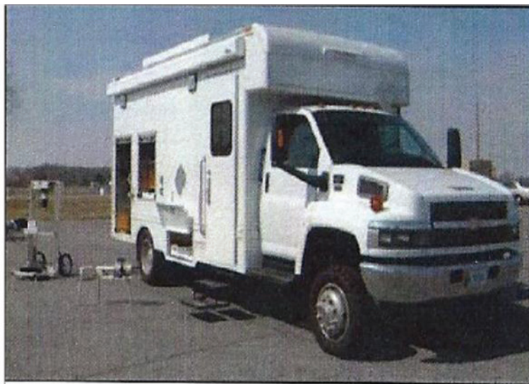
FIGURE 4-3 Mobile munitions assessment system. Contents include heating and air conditioning system; electrical power supply and distribution system; PINS system; radiography systems; Raman spectroscopy system; data acquisition and handling system; audio/video equipment; communications equipment; and support equipment. SOURCE: Laurence G. Gottschalk, PMNSCM, “Program Status and Update to NRC,” presentation to the committee on September 27, 2011.
