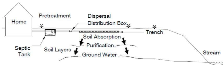
FIGURE 2-5 Idealized individual on-site sewage treatment and disposal system flow diagram.
