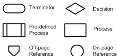
In each of the figures, common flow charting symbols are used. Rectangles represent processes, diamonds represent binary decision points (yes or no), while ovals represent terminal points in the process—a beginning or an ending. Circles and pentagons transfer the reader to other points in the processes where the next sequential step occurs if it does not directly follow the previous step in the overall process.
