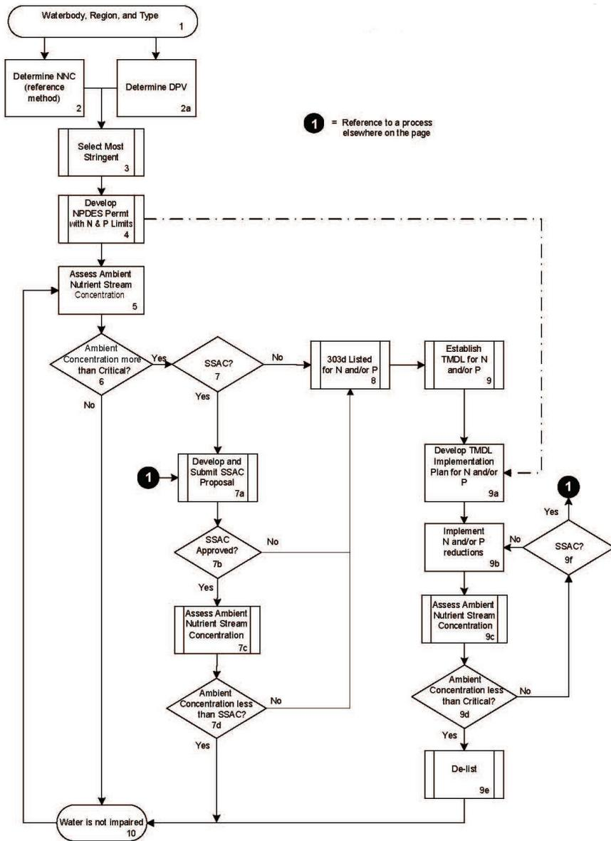
FIGURE A-2 Process for Numeric Nutrient Criteria in Flowing Waters
