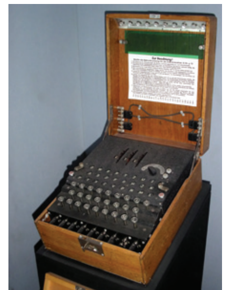
6 / The World War II-era Enigma is one of the most well-known examples of cryptography machines and was used to encrypt and decrypt secret messages. Photo by Karsten Sperling. /
