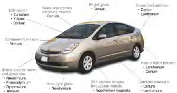
FIGURE 2-4 New hybrid vehicles incorporate many critical elements.
