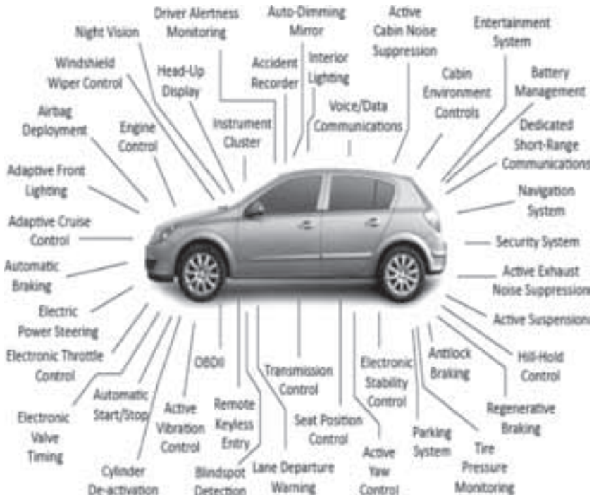
FIGURE 2-1 Types of electronics systems in modern automobiles. (Source: Clemson University Vehicular Electronics Laboratory.)
