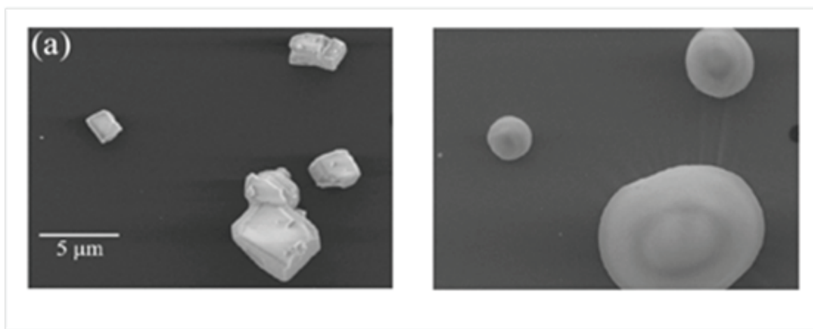
FIGURE 4-5 Calcium carbonate particles react with nitric acid in the presence of water vapor. SOURCE: Grassian, 2010.
