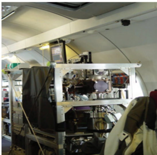
FIGURE 3-2 SPLAT II, an ultrasensitive high-precision instrument for multidimensional single particle characterization. SOURCE: Zelenyuk, 2010; modified from Zelenyuk et al., 2009.
