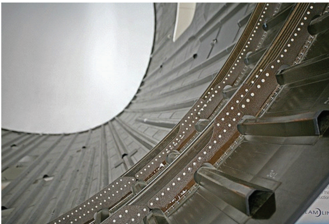
FIGURE 2-18 787 composite fuselage structures. SOURCE: Justin Hale. 2006. “787 from the Ground Up.” Aeromagazine . The Boeing Company, Quarter 4. Pp. 16-23.
