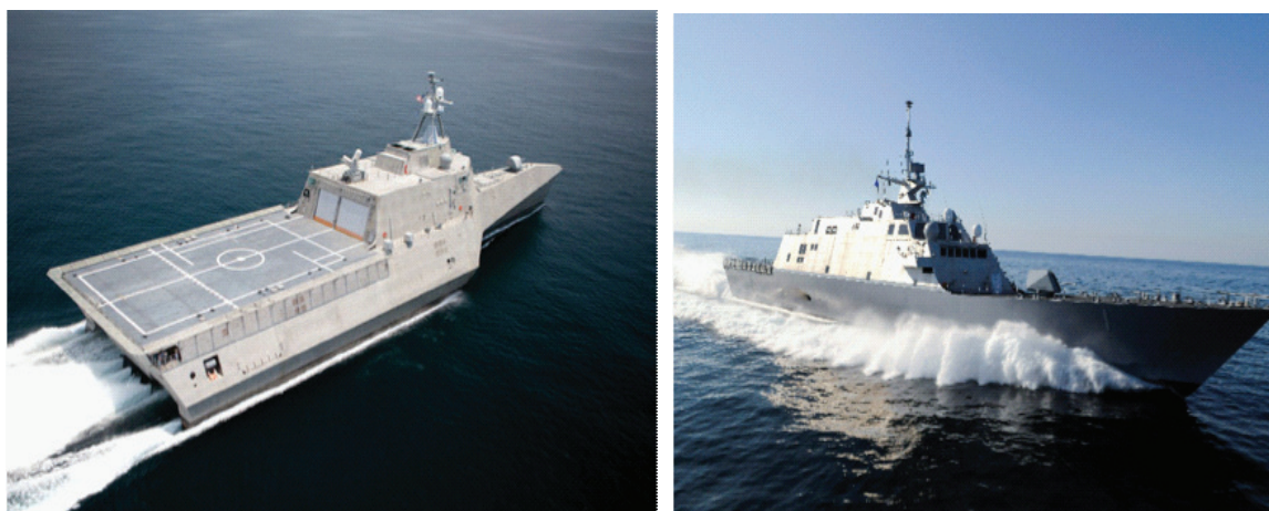
FIGURE 3-8 Littoral combat ship trimaran (Austal USA—left) and monohull (Lockheed Martin—right). SOURCE: CAPT Mike Good, Program Manager LCS Mission Modules, “Littoral Combat Ship (LCS) Program Overview,” Northwest Florida Defense Coalition, May 14, 2009.
