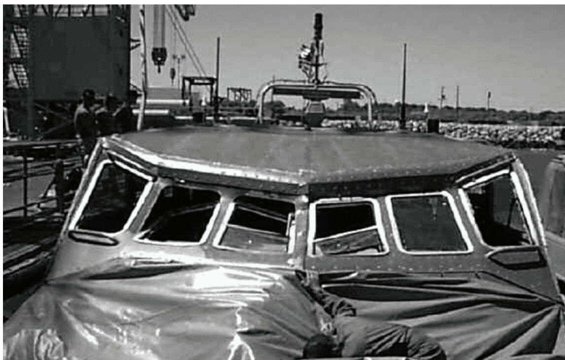
FIGURE 3-6 Wave damage to Mark V special operations craft. SOURCE: J. Grimsley and E.G. Hatchell. 2008. “Computational Tools for Combatant Craft.” NSWCCD, SeaFrame , Vol. 4, Issue 2.
