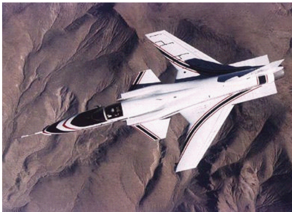
FIGURE 2-15 X-29 aircraft, featuring forward-swept wings. SOURCE: NASA Dryden Flight Center Photo Collection, available at http://www.nasa.gov/centers/dryden/images/content .
