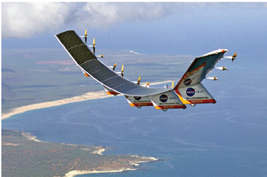
FIGURE 2-13 NASA's HELIOS, a type of high-altitude long endurance (HALE) vehicle. SOURCE: NASA Dryden Research Center Photo Collection, available at http://www.nasa.gov/centers/dryden/images/content/105841main_helios.jpg .
