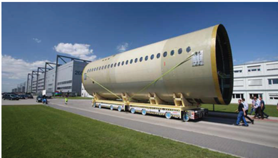
FIGURE 2-19 Test fuselage section for the Airbus A350 XWB aircraft. SOURCE: Airbus.
