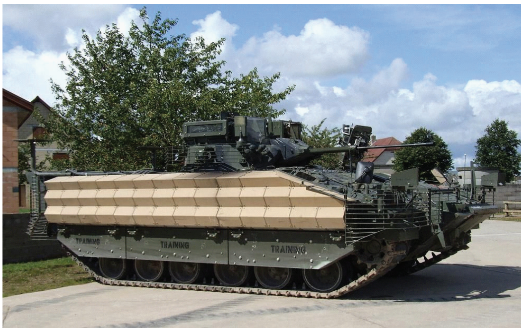
FIGURE 4-1 A warrior vehicle with added reactive appliqué and bar-armor. SOURCE: BAE Systems, U.S. Combat Systems, “Lightweighting in Military Vehicles,” presentation to the committee, December 8, 2010.
