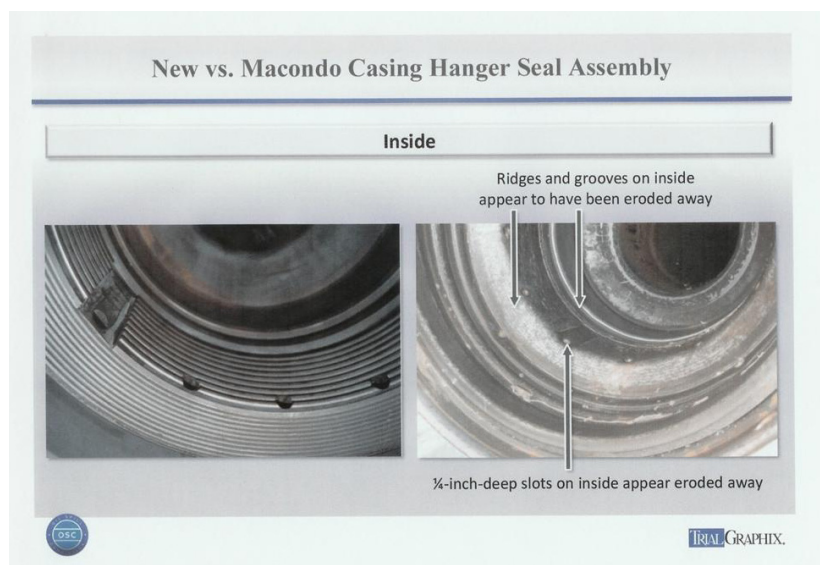
FIGURE 2-9 View inside casing hanger. Source: Presidential Commission 2010, Slide 118.
