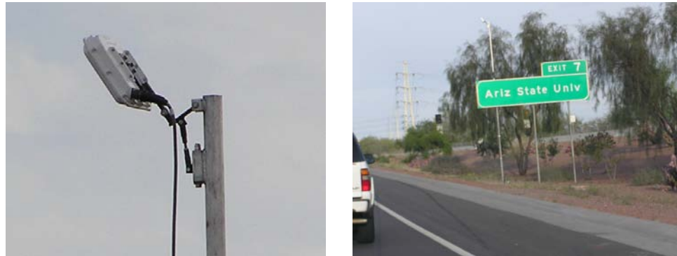
Exhibit 3-10 Side-Mounted Digital Wave Radar Used by TRA for Data Collection. Left photo: Close-up view of the radar unit. Right photo: Radar unit collecting data at EN-EN site.
