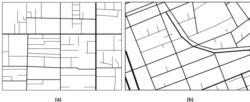
FIGURE 7 Maps showing (a) a more “organic” area with a majority of three-way intersections, although major roads have been widened and straightened, and (b) an area with some three-way intersections, but overall greater organization, or planning of all roads. Both images are drawn to the same scale and are roughly 400 m by 300 m.
