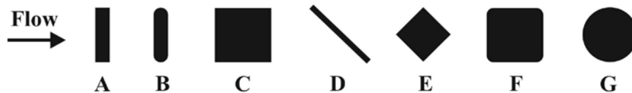
Figure 4-8 Cylinders differing in cross-sectional shape, but having the same projected width to the flow (Mostafa 1994)
