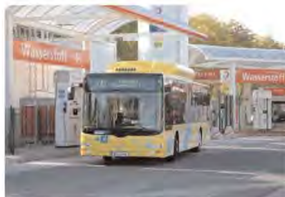
A HICE bus at a refueling station in Berlin, Germany (Source: HyFLEET:CUTE Website).
