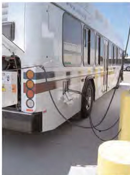
A fuel cell bus at Santa Clara VTA is filled with compressed hydrogen.
