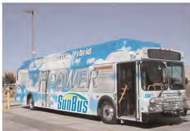
A 40-ft hybrid-electric HICE bus, operated by SunLine Transit in Thousand Palms, California
