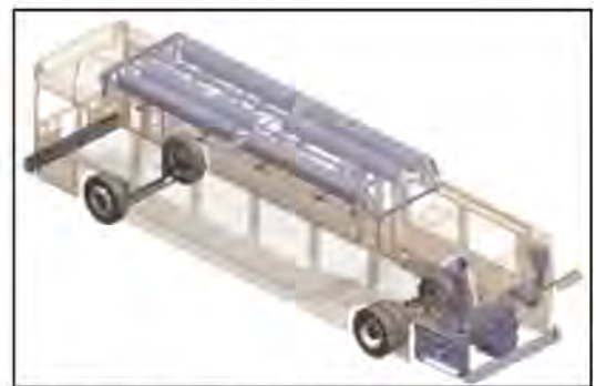
CNG bus overhead storage tank placement (Source: New Flyer Website)
