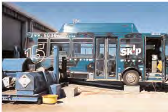
A CNG bus from Boulder, Colorado, is emissions tested on the WVU transportable dynamometer.
