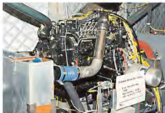
A Cummins diesel engine converted to run on DME (Source: Transport Canada Website).
