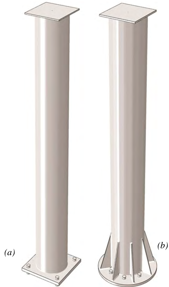
Figure 70 Global model of analyzed structures: (a) with unstiffened tube-to-transverse plate connection; (b) with stiffened tube-to-transverse plate connection
