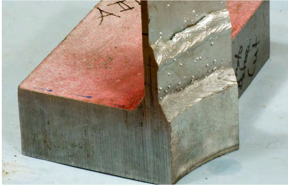
Figure 153 Lack of fusion at the backing ring-to-tube weld
