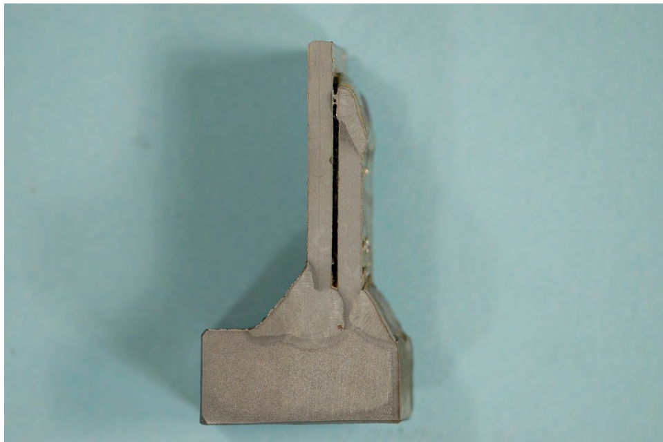
Figure 154 Polished and etched section showing lack of fusion at the backing ring-to-tube weld (Figure 153)
