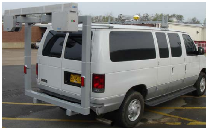
FIGURE 8 Implementation of LRIS into a highway data vehicle.
