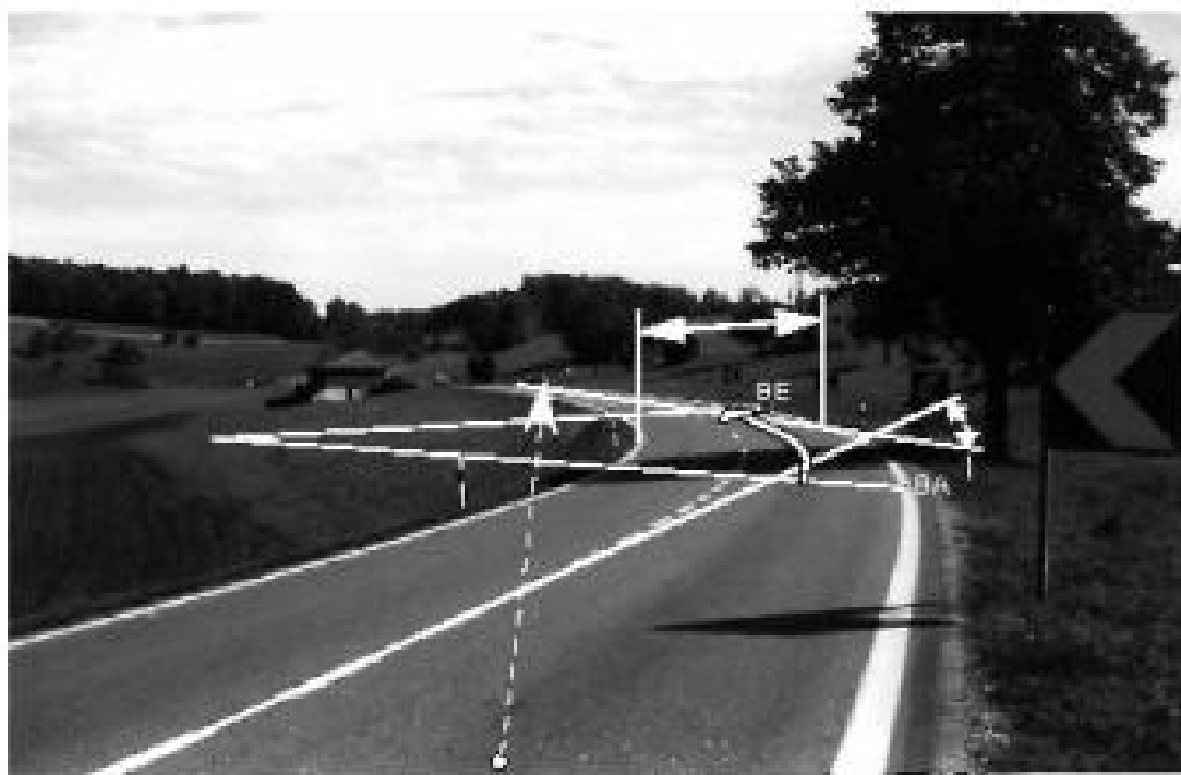
FIGURE 10 Curve parameters found to significantly influence operating speed in curves.
