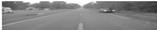
Figure A.13. Identification of intentional lane departure for vehicle parked on shoulder: (a) vehicle wheel path shows lane departure and (b) video indicates lane departure was the result of the subject vehicle moving over for parked vehicle.
