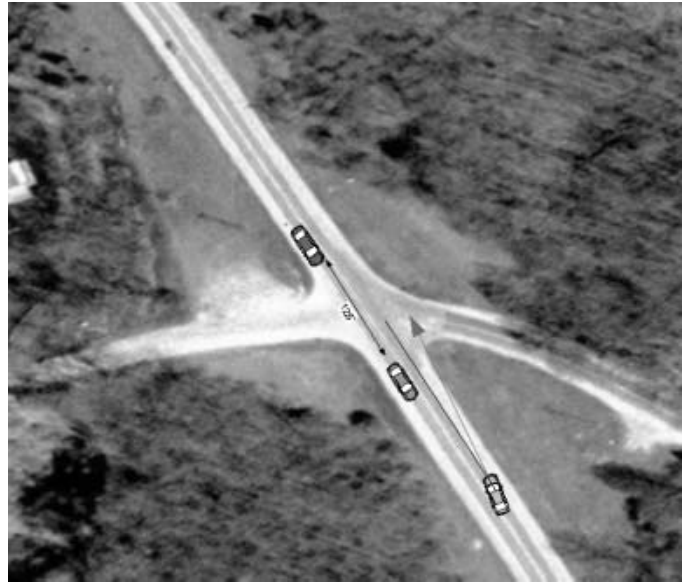
Figure 5.15. Schematic of a vehicle departing its lane and its likely path if the driver does not correct lane departure.
