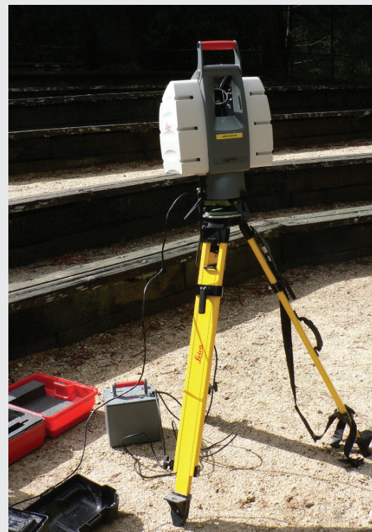
Leica HDS-3000 terrestrial lidar scanner.
