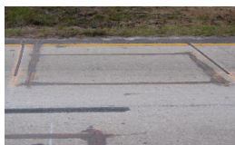
In 2001, data from the Florida pilot site were collected with ceramic piezoelectric sensors ( above ) and in 2005 with quartz piezoelectric sensors ( below ).
