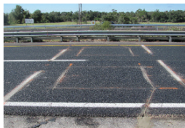
In 2001, data from the Florida pilot site were collected with ceramic piezoelectric sensors ( above ) and in 2005 with quartz piezoelectric sensors ( below ).
