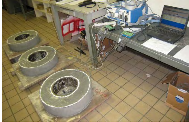
Figure 11.3.7: AASHTO PP34 test setup
