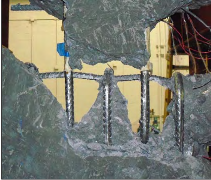
Figure 9.2.22: Deformation of lacer bar
