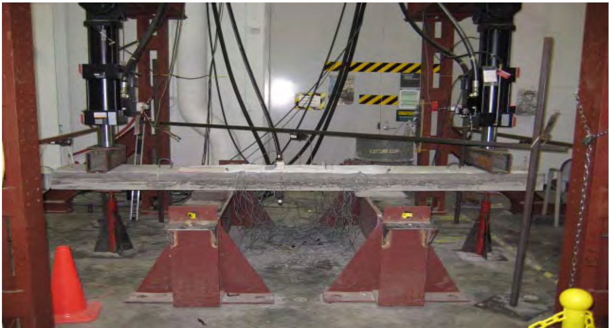
Figure 9.1.5: Flexural test set-up (Longitudinal Joint Test)
