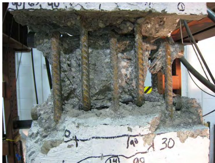
Figure 13.1.15: Deformation of lacer bar
