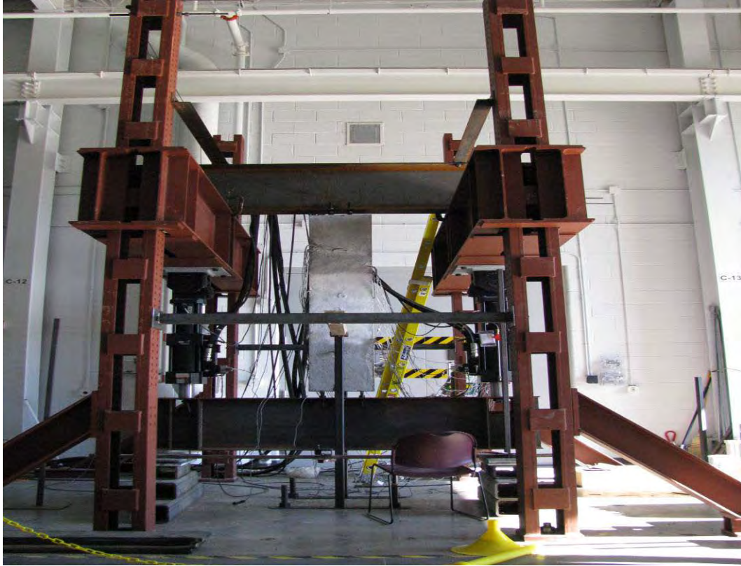
Figure 9.1.6: Tension test set-up (Transverse Joint)
