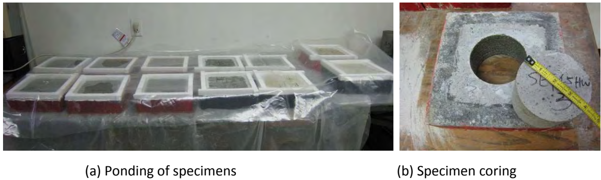
Figure 11.3.3: Specimen preparation per ASTM C 1543
