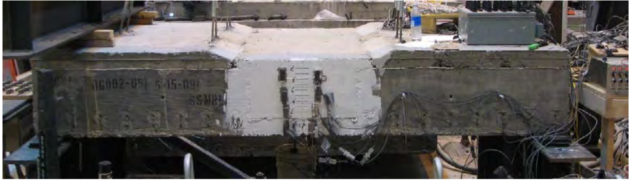
Figure 6.1.5: Elevation view of SSMBLG3-HighBars and increased deck depth to provide additional cover for the shrinkage reinforcement in the deck
