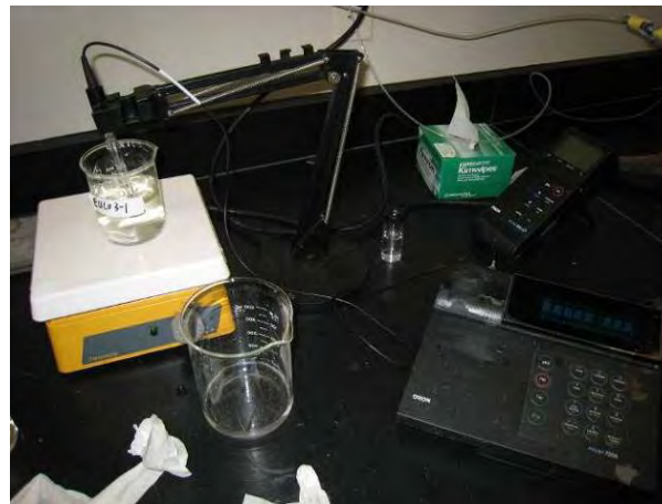
Figure 11.3.4: Chloride concentration determination with ISE
