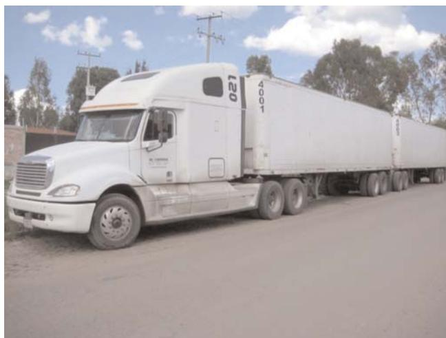
**Figure 5** T3-S2-R4 LCV used in Mexico.
