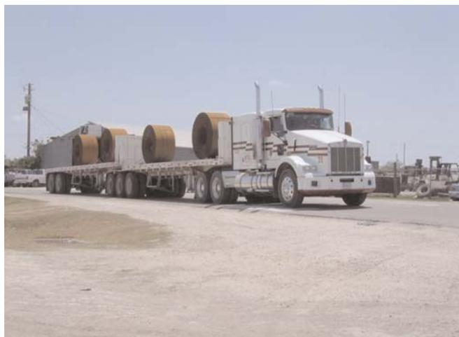
**Figure 6** T3-S3-S2 LCV used in Mexico.
