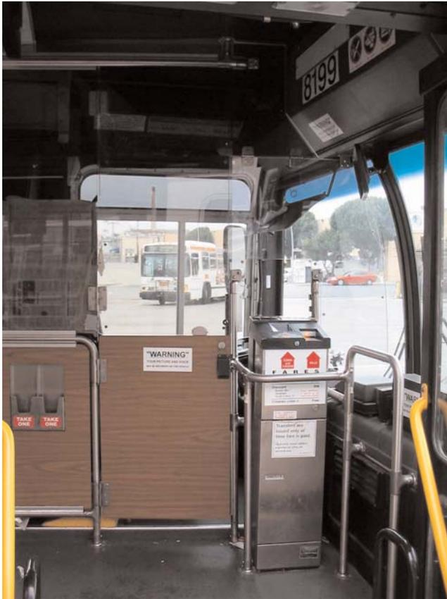
FIGURE 15 SF MUNI barrier. (Courtesy: SF MUNI.)
