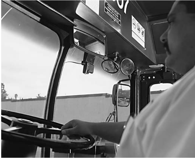
Figure 13. Video data recording system installed behind rearview mirror in a transit bus (photo courtesy of DriveCam, Inc.).
