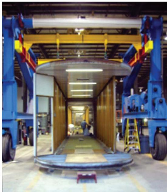
FIGURE 35 Tami-Lift mobile gantry crane.
