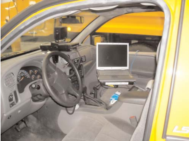
FIGURE 27 In-vehicle FOD documentation system. Source: Paul Khera, Alaska Department of Transportation.
