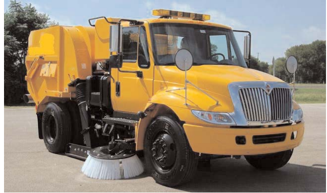
FIGURE 22 Vacuum with mechanical broom and regenerative air feature. Source: Tymco.
