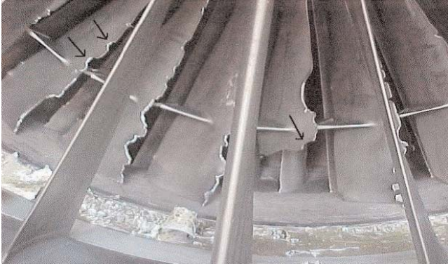
FIGURE 1 Results of engine ingestion of FOD. Source: Jim Stephan, Delta Air Lines Corporate Safety, Oct. 25, 2005, FOD/Wildlife, An Airline's Perspective presentation. [Online]. Available: http://www.fodnews.com/FOD_For_FAA-gif/slide001.htm .
