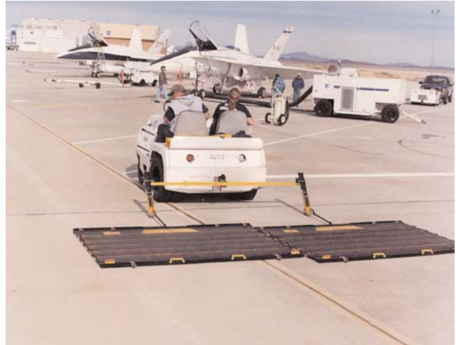
FIGURE 14 Tow-behind friction mat. Source: Sherwin Industries.
