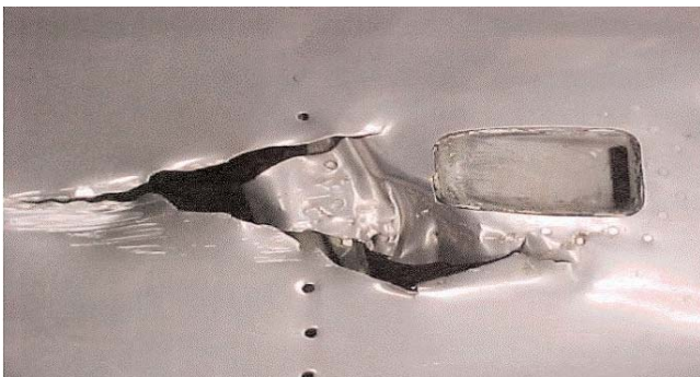
FIGURE 2 Result of fuselage damage from FOD. Source: Jim Stephan, Delta Air Lines Corporate Safety, Oct. 25, 2005, FOD/Wildlife, An Airline's Perspective presentation. Available: http://www.fodnews.com/FOD_For_FAA-gif/slide001.htm .
