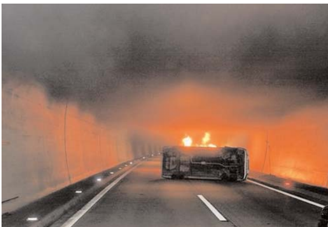
FIGURE 10 Plabutch Tunnel Fire Test sponsored by Graz University of Technology.
