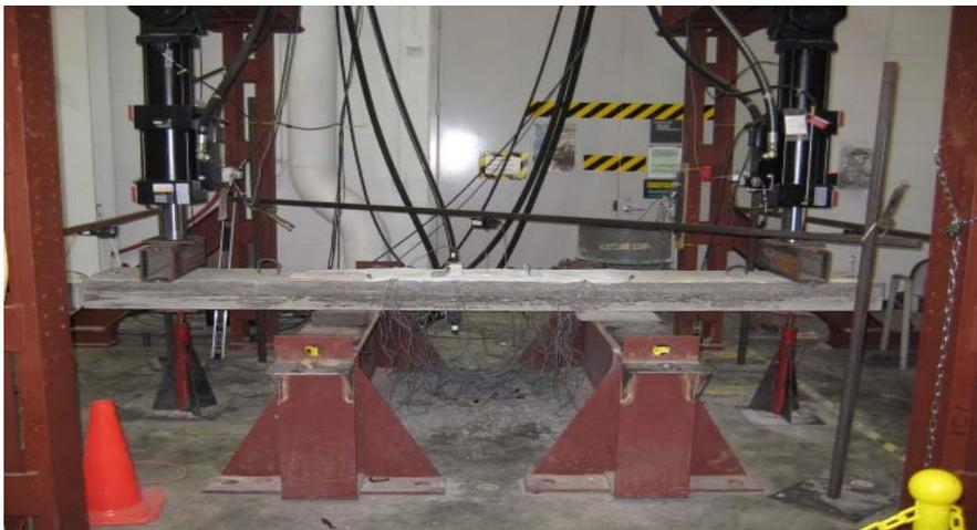
**Figure 18** Flexural test set-up (longitudinal joint test) (LVDT = linear variable differential transformer).
