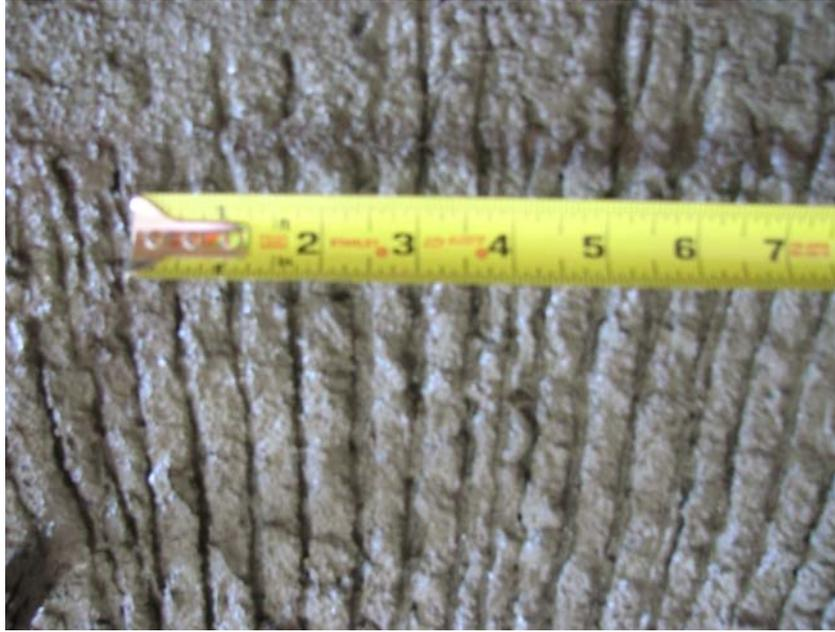
**Figure 13** Intentionally roughened surface, by means of raking, of top web of precast beam used for the construction of Concept 2 laboratory bridge specimen.
