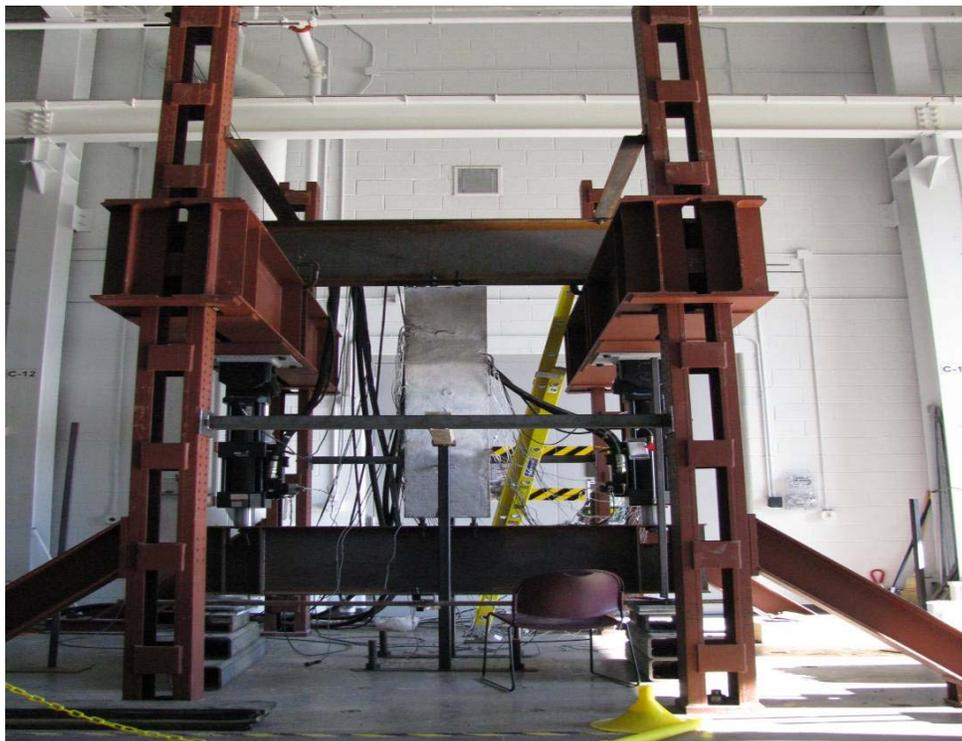
**Figure 19** Tension test setup (transverse joint).
