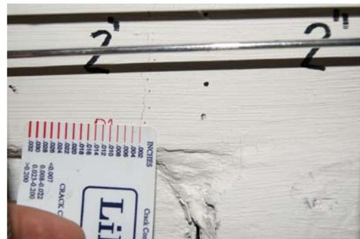
**Figure 8** Measurement of width and length of crack observed on origin and end faces of subassemblage specimens.
