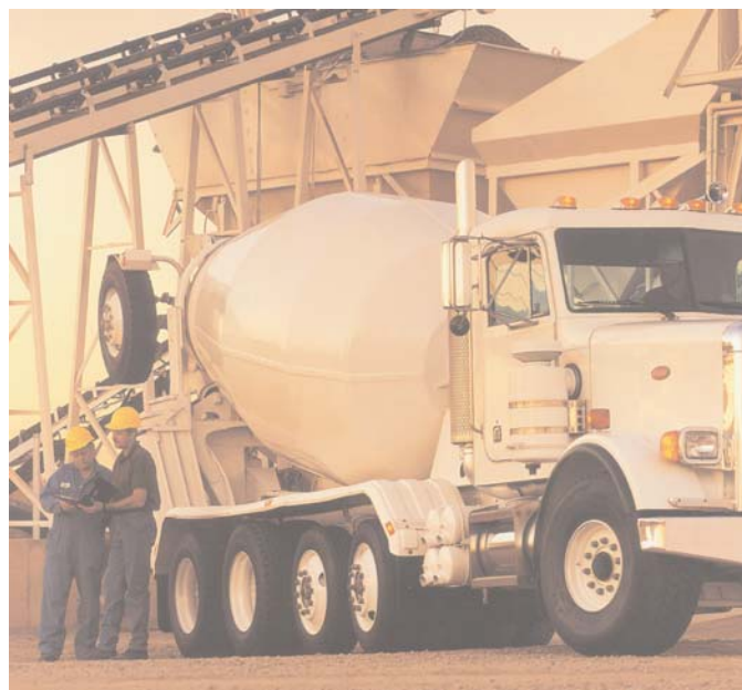
Figure 6. Concrete ready-mix truck with quad axle.
