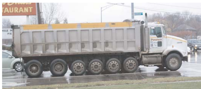
Figure 7. Multi-axle specialized hauling vehicle (Sivakumar et al. 2007).
