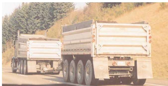
Figure 8. Truck with tridem and quad axles.
