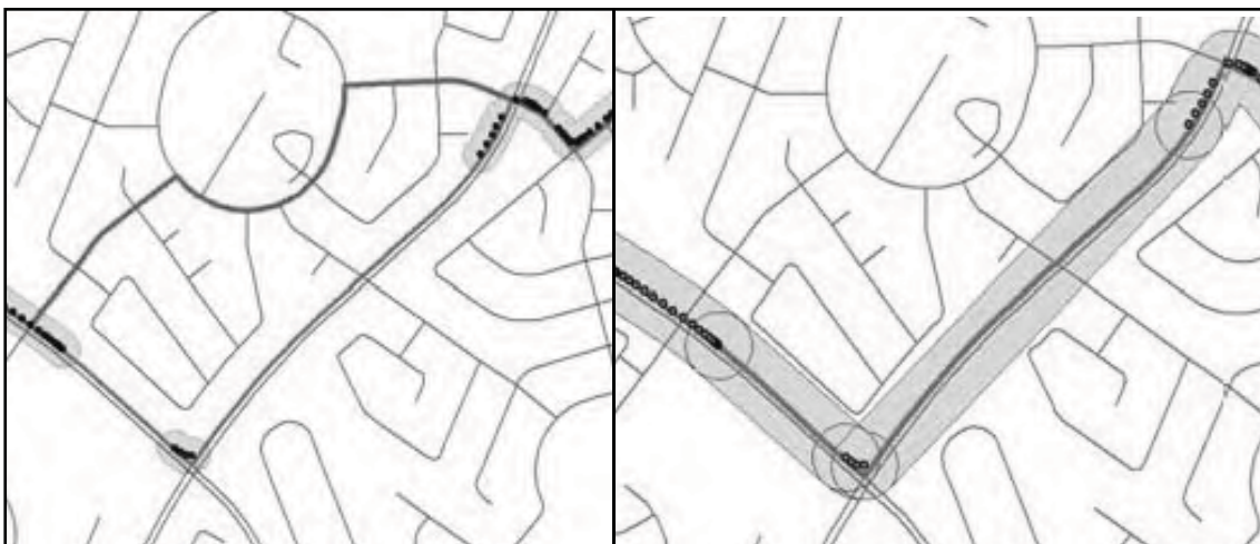
Figure 7.4. GPS gaps: (left) before links added; (right) after links added.
