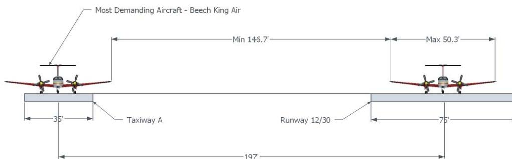
Figure H-20. Cross-section of the existing separation at TAN.
