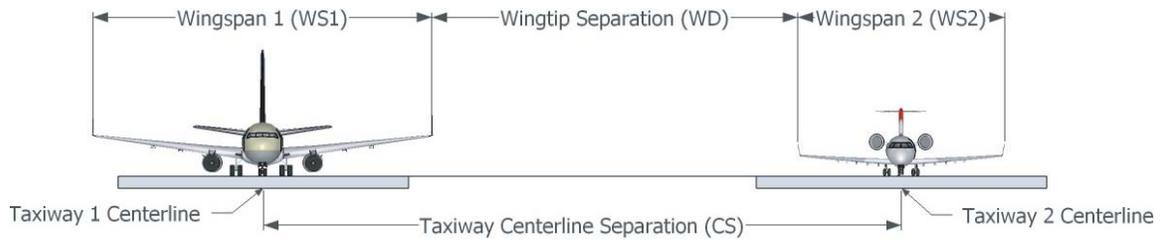
Figure A-2. Example of taxiway/taxiway separation analysis for specific aircraft.
