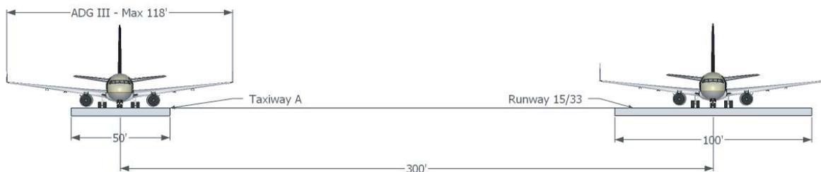
**Figure H-3. Cross-section of the existing separation at ADS.**
