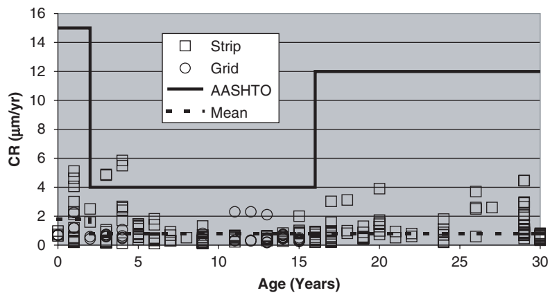
Figure 11(b). Corrosion rates vs. time and comparison with the AASHTO model for galvanized elements within high quality fill.
