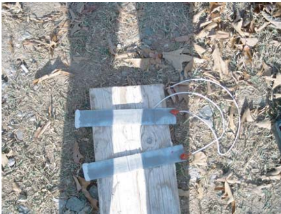
3. Galvanized coupons prepared for installation
